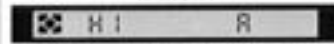
Overexposure; select smaller aperture setting (larger f number) or use Nikon ND filter
